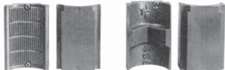
Dies with full circle contact for running tubing.
