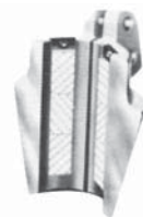
Type "TD" Slips with replaceable "Chevron" inserts. Inserts have 35% greater contact than the Circular Button type. Recommended for the heavier tubular string load. Available for either single or parallel strings operation. (Fig. 8)
